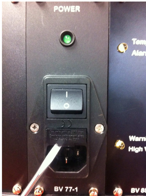
Fig 9: Location of the main power supply fuse
