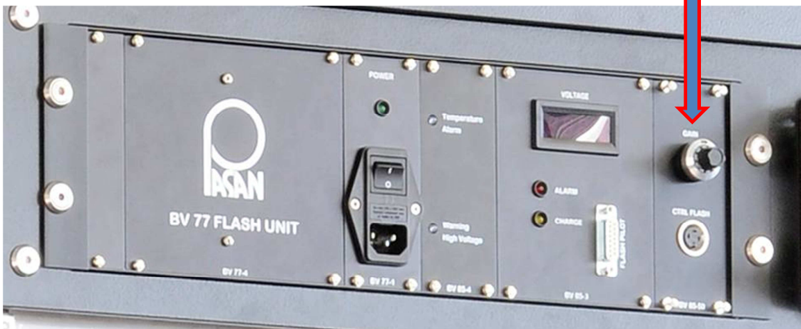
Fig 4: electronic cards on the flash generator
